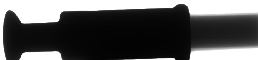
Figure 5 DR detection at the end of composite insulator (55 kV, 3 mA)
