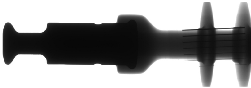
Figure 6 DR detection at the end of composite insulator (60 kV, 2 mA)
