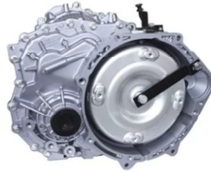
Figure 2(a). The detail information of WLY·CVT25
