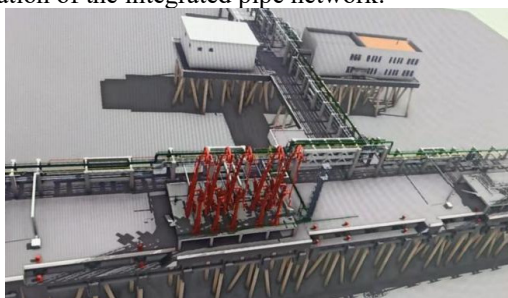
Fig6. Dynamic simulation screenshots of pipes installation
