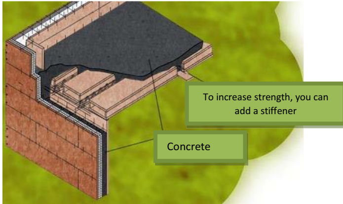
Fig. 4. VELOX - technology of low-rise civil construction
