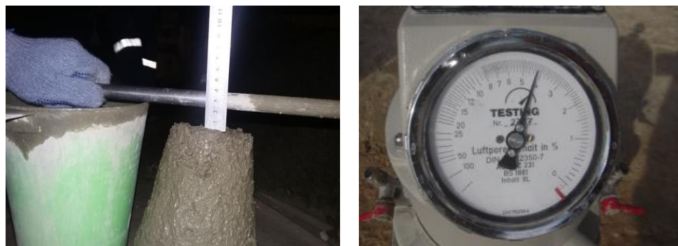
Fig. 4. The process of determining the basic properties of cement concrete mix
