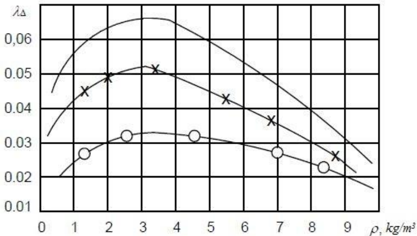
Fig. 6. Change in the coefficient of hydraulic resistance of a turbid flow depending on the concentration of suspended sediment \rho according to the Peoples' Friendship University named after P. Lumumba [19].
