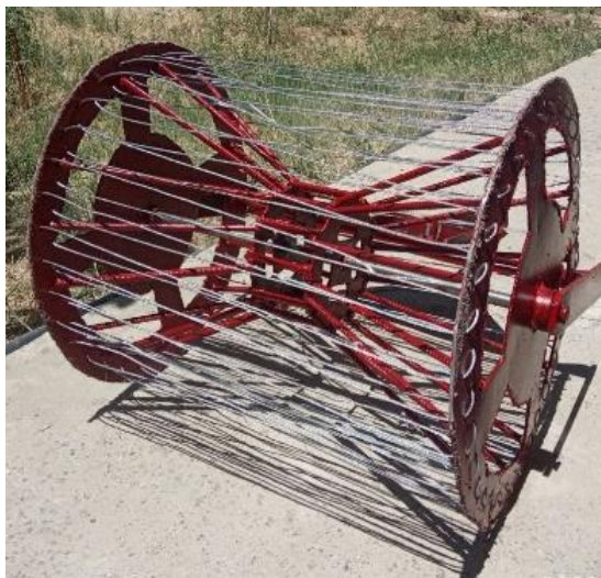
Fig. 1. General view of the working body of the comb-forming machine with elastic rods
