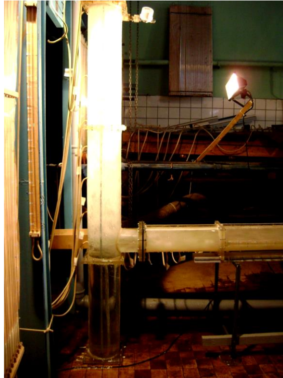
Fig. 25. Pattern of water flow in the abutting zone of the outlet tunnel to the shaft at a maximum flow rate Q=3130 \text{ m}^3/\text{s} and air supply Q_a=67 \text{ m}^3/\text{s}
