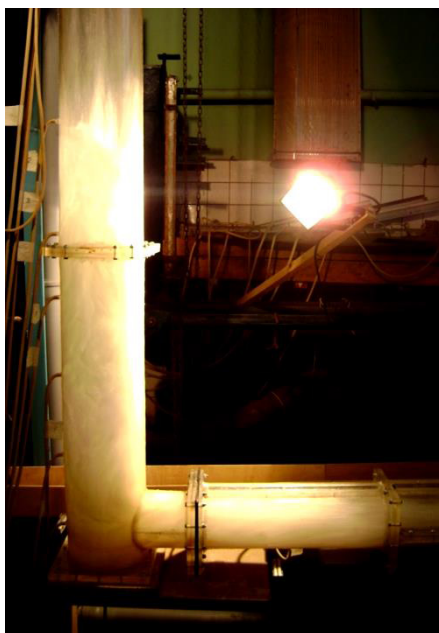
Fig. 16. Initial section of the tunnel at a flow rate Q=2300\text{m}^3/\text{s} when a/a_o=1.0 and the air is supplied At the outlet section, a flow is formed with a rather steep drop-down curve, when a critical depth is formed in the outlet section, slightly more than half the tunnel diameter, as can be seen from Figure 17.
