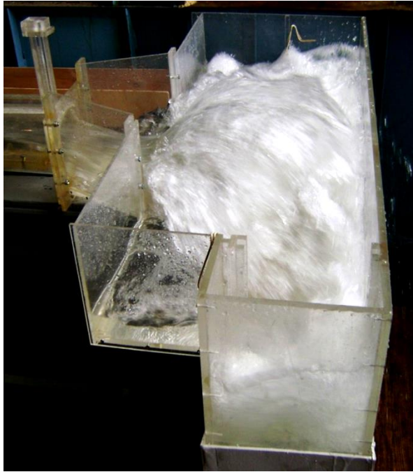
Fig. 17. Outlet section of the outlet tunnel at a flow rate Q=2300 \text{ m}^3/\text{c} when a/a_0=1.0 and the air is supplied
