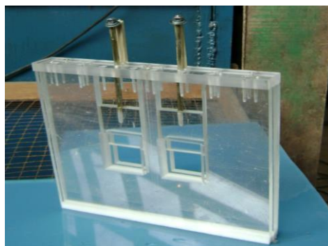
Fig. 9. Design of the shutter chamber with two shutters with a sharp edge
