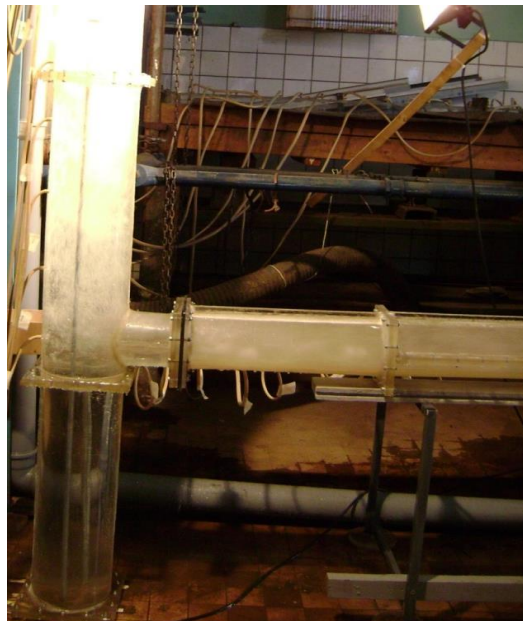
Fig. 23. Pattern of water flow in the abutting zone of the outlet tunnel to the shaft at Q=2650\text{m}^3/\text{s} and air supply Q_a=50\text{ m}^3/\text{s}
