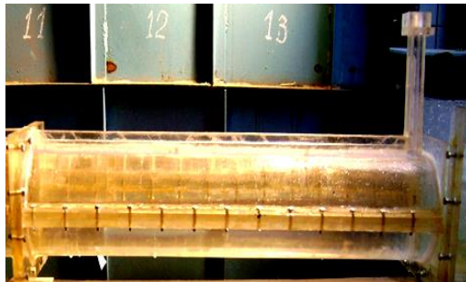
Fig. 25. Pattern of water flow in the abutting zone of the outlet tunnel to the shaft at a maximum flow rate Q=3130 \text{ m}^3/\text{s} and air supply Q_a=67 \text{ m}^3/\text{s}
