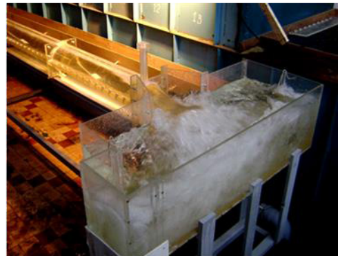
Fig. 25. Pattern of water flow in the abutting zone of the outlet tunnel to the shaft at a maximum flow rate Q=3130 \text{ m}^3/\text{s} and air supply Q_a=67 \text{ m}^3/\text{s}
