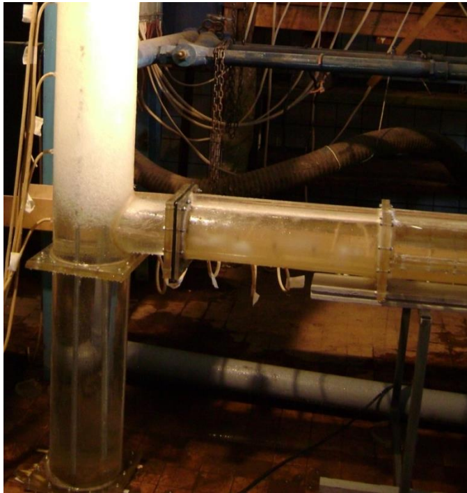
Fig. 20. Movement of water in the abutting zone of the outlet tunnel to the shaft at Q=630\text{m}^3/\text{s} and air supply Q_a=11\text{ m}^3/\text{s} .
