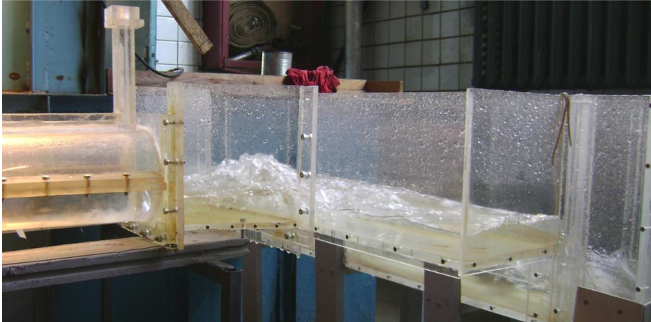
Fig. 22. Pattern of water flow at the end section of the outlet tunnel when air is supplied Q_a=11\text{ m}^3/\text{s} , Q=630\text{ m}^3/\text{s}
