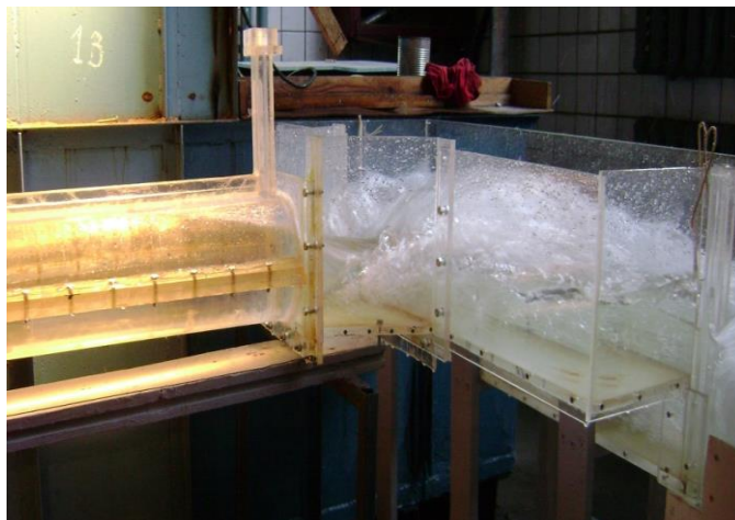
Fig. 24. Pattern of water flow in the area of the end section of the tunnel at Q=2650 \text{ m}^3/\text{s} and air supply Q_a=50 \text{ m}^3/\text{s}
