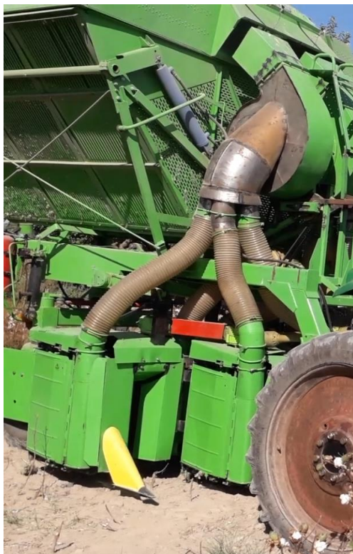
Fig. 1. Pneumatic system of the vertical-spindle cotton harvester MX-2.4
