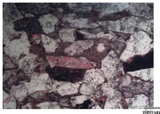
c. Well C, Chang 6, intragranular dissolved pores and residual intergranular pores, single polarized light, cast body sheet
