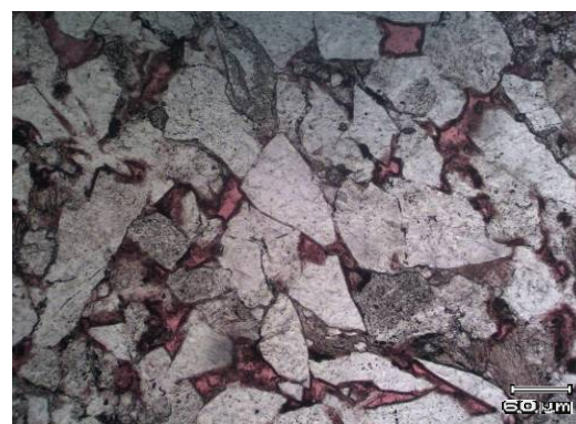
a. Well A, Chang 6, residual intergranular pores, single polarized light, cast body piece
