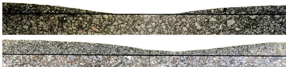
Fig. 2. Abrasive wear of the road surface in the Kazan.
