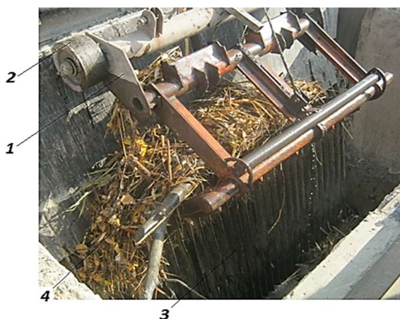
Fig. 3. The process of covering the mouths: 1 – device base; 2 – device base wheels; 3 – grid holding traps; 4 – a set of mouthpieces with different contents.
