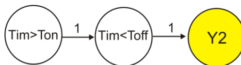
Fig. 2. Lighting control graph-diagram.
