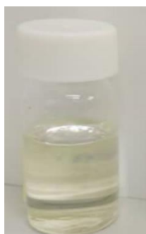
Figure 1. Successful DES 2 obtained when menthol and butanoic acid are combined with 1:1 molar ratio.
