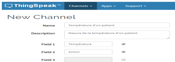
Fig. 4. Window to create channel and fields on Thingspeak.com site
