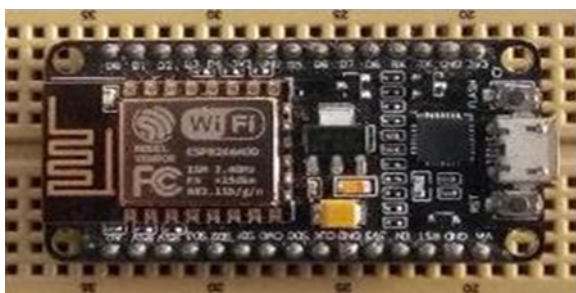
Fig. 1. The image and main characteristics of the NodeMcu used
