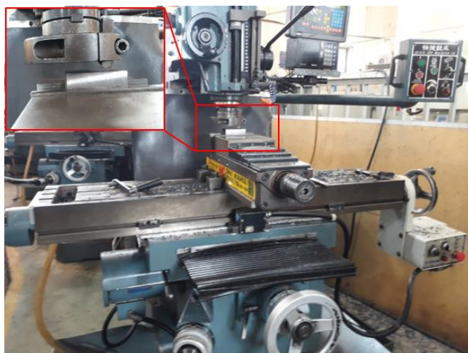
Fig. 1. JL VH320B vertical milling machine
