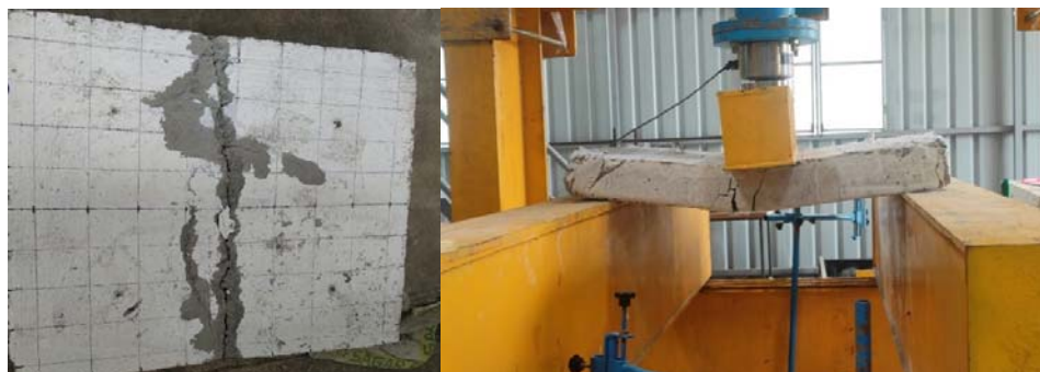
Fig.5. Testing of slab specimens
