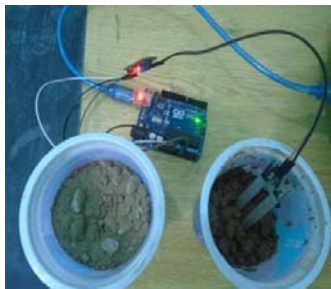
Fig. 5. IoT Moisture Content testing.
