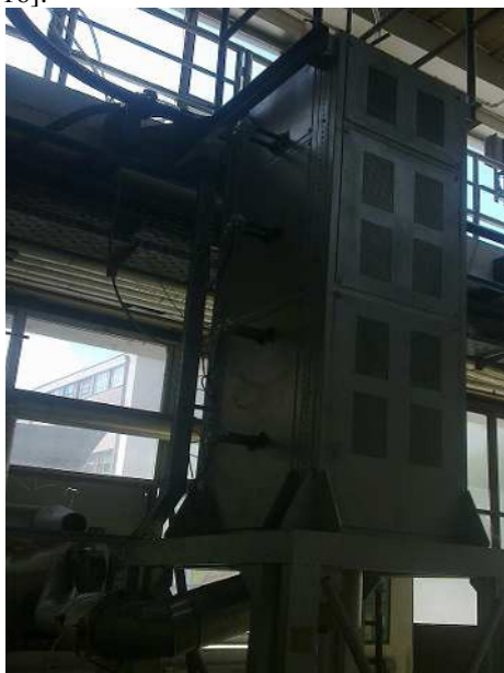
Figure 1. AUCR experimental line: front view of four visible zones with temperature measurement of the reaction tube and process control
