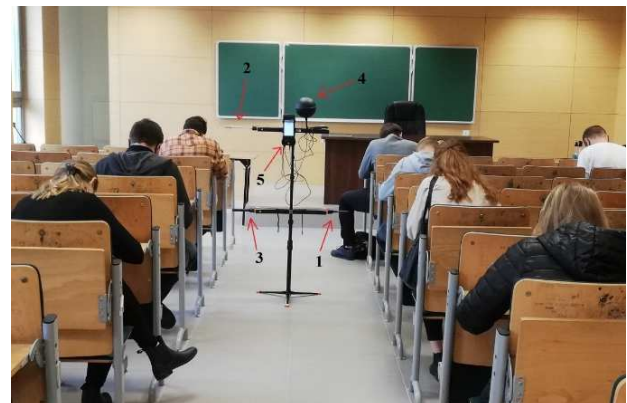
Fig. 2. Photo of the test stand with the Testo 400 microclimate measuring device in the test room.
