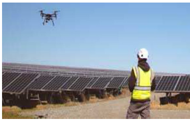
UAV-based infrastructures inspection
