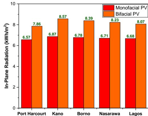
**Figure 4** Single Day In-Plane radiation on Monofacial and Bifacial PV modules in the various climatic region for August
