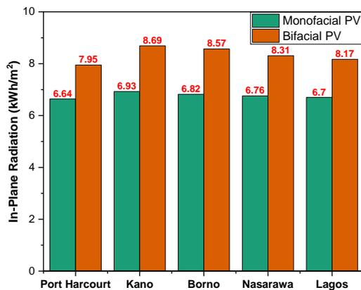
**Figure 3** Single Day In-Plane radiation on Monofacial and Bifacial PV modules in the various climatic regions for April
