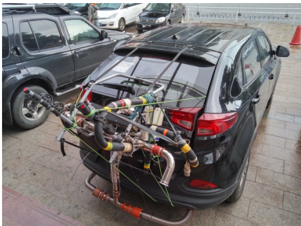
Fig. 2. Installation statuses of test apparatus in vehicle 1 for RDE tests.
