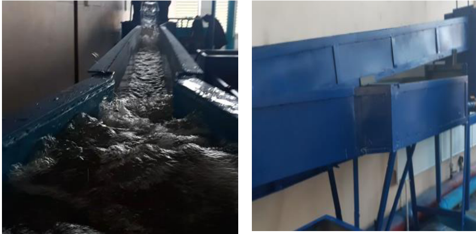
Fig. 6. Side outlet water well model.
