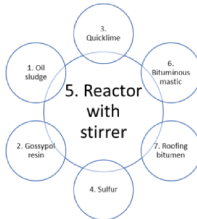
Fig. 3. Scheme for obtaining a bitumen-replacing mixture for the use of insulating and roofing coatings: 1. OS-oil sludge; 2. GR - gossypol resin; 3. Q - quicklime; 4. S - sulfur; 5. Reactor with stirrer; 6. BM - bituminous mastic; 7. RB - roofing bitumen.
