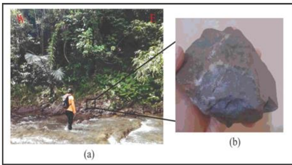
Fig. 4. Outcrop of altered andesite unit at the research area (a) and hand specimen of altered andesite rock sample (b)
