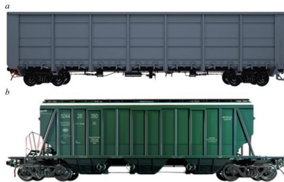
Fig. 3. General view of the innovative gondola wagon model 12-9853 (a) and the innovative hopper wagon for grain transportation model 19-9870-01 (b)
