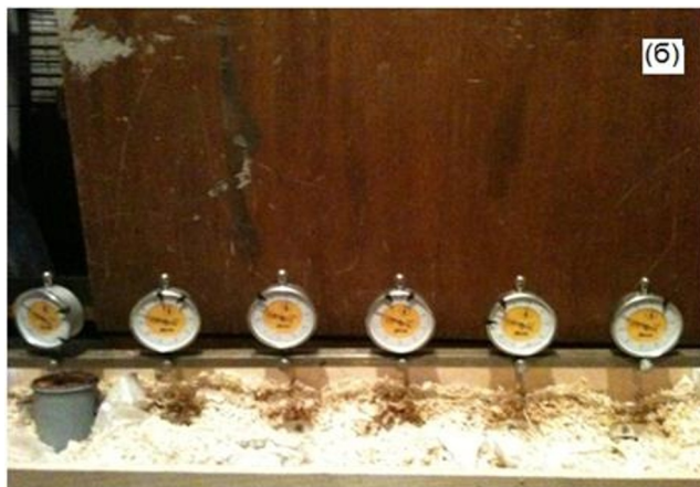
Fig. 1. General view of the installation for determining heaving under conditions closed system.
