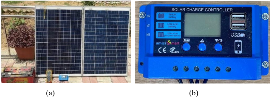
Fig. 2. (a) Solar Panels used in the implementation of the project (b) Solar Charge Controller
