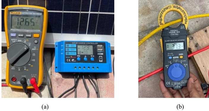
Fig. 5 (a) Battery Output terminals (In multi-meter), (b) Total Output current of the system
