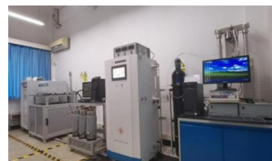
Figure 1 Stress sensitive nuclear magnetic resonance testing device
