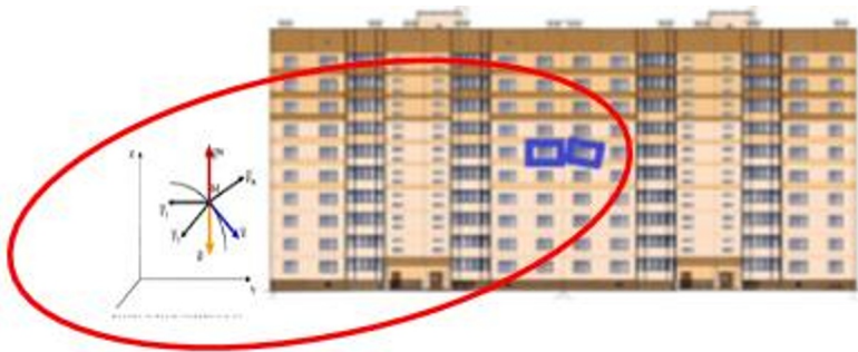
Fig. 2. Scheme of possible vibration vibrations of structural elements relative to each other, and relative to the skeleton of the building.
