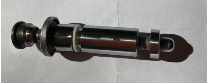
Fig. 1. Axial piston pump plunger with fluoroplastic seal
