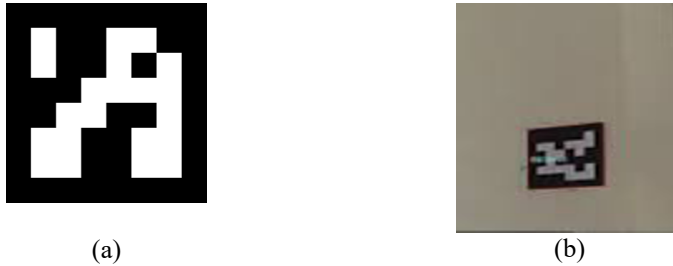
Figure 4. (a) Marker Aruco (b) Marker Aruco installed in wall
