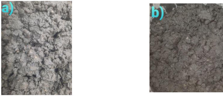
Fig. 2. View of basalt-fiber concrete mix after discharge from the mixer. (a) - using the first method; (b) - the same, using the second method.
