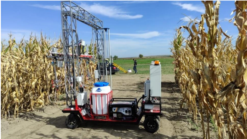
Fig. 3. Autonomous robot for plant protection
