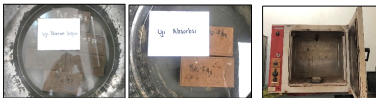
a) Soaking in sodium sulphate solution b) Soaking in water for absorption test c) Drying of test objects
