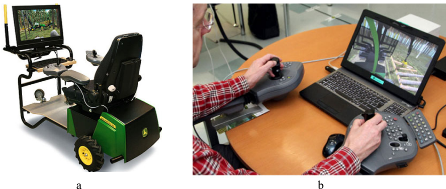
Fig. 2. Logging equipment simulator: a – 3D simulator; b - personal computer simulator.
