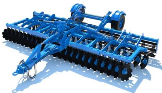
Fig. 1. Disk harrow BDP-6×2P of CJSC Rubtsovsky Spare Parts Plant.
